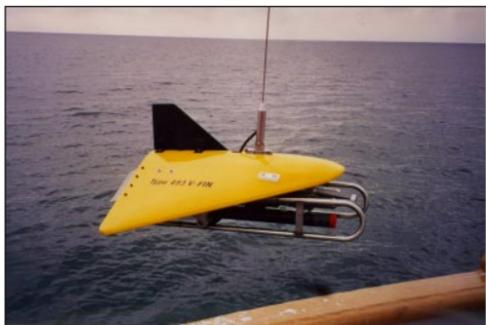
Figure 1. The plankton survey system being put over the side of a research vessel.
